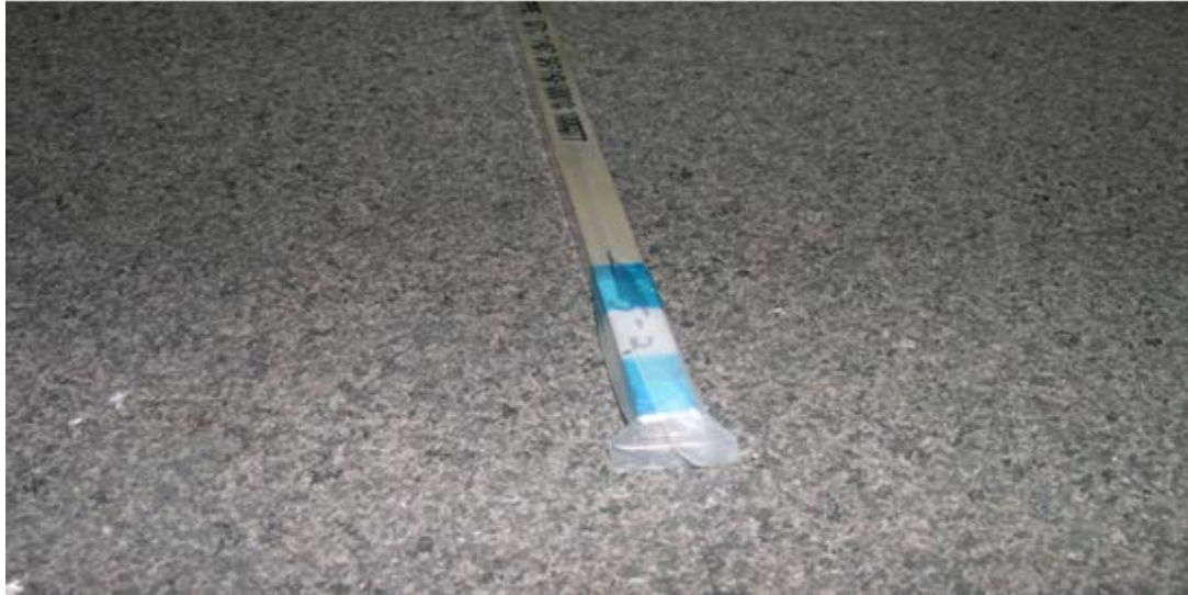
Figure 3. FOIL PROTECTED EXTRUSION WITH POLY SLEEVE TAPED ENDS
