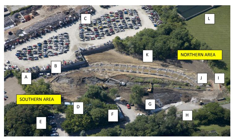
SOUTH EXCAVATION AREA (9.1.09) - (A) Haley's Ditch Starting Point; (B) Bypass pump (C) LKQ Property (D) Water Treatment System (E) Contractors' Parking Area (F) Office Trailer (G) Stockpile (H) Truck Loading Area (I) Temporary Bridge (J) Bypass Pump Discharge (K) Temporary Overflow Channel (L) IRG Property
