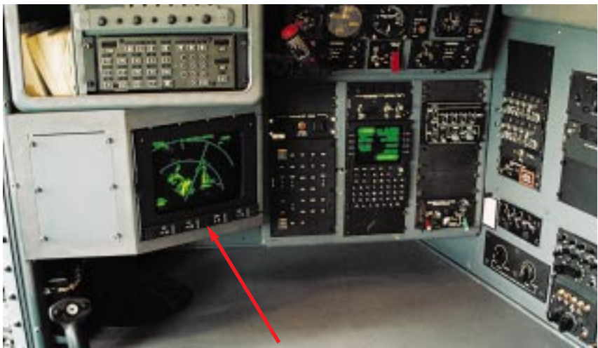
The AN/APN-241 Navigator Display in a C-130H aircraft.
