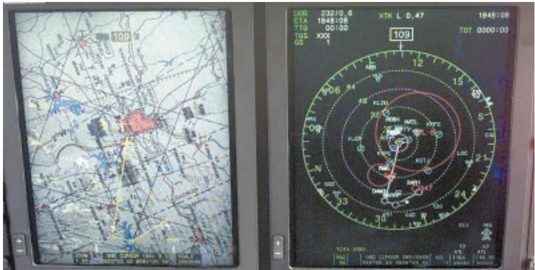
The C-130J Head Down Displays of the Digital Moving Map presentation on the left and the Centered Format Nav/Radar Display on the right with Flight Plan, Airports, Nav Aids, Radar Warning Receiver, and Tactical Plot overlays.
