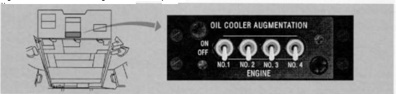
Figure 3. Overhead oil cooler augmentation control panel.
