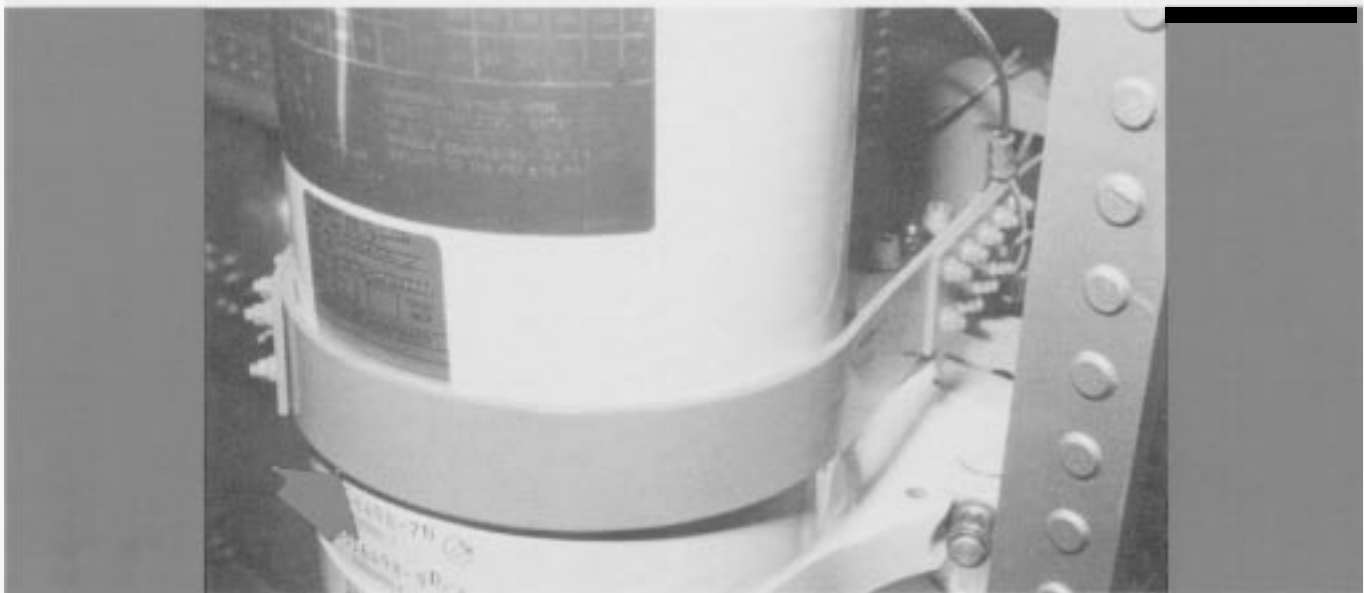
Figure 4. The tiedown fixture strap in position, as seen from the MLG wheel well.
