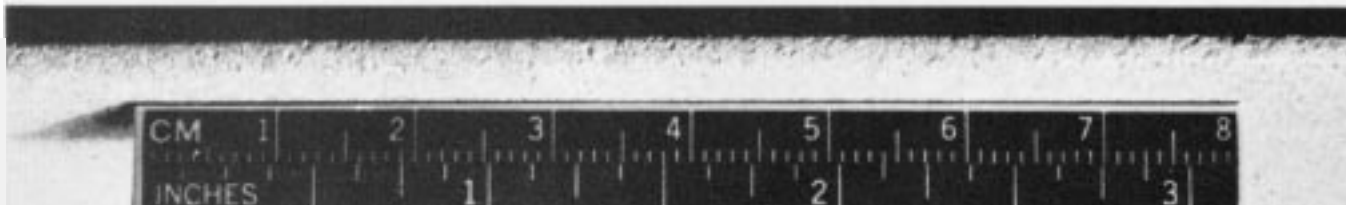
This blade leading edge is in need of rework. Note coarse surface texture.
