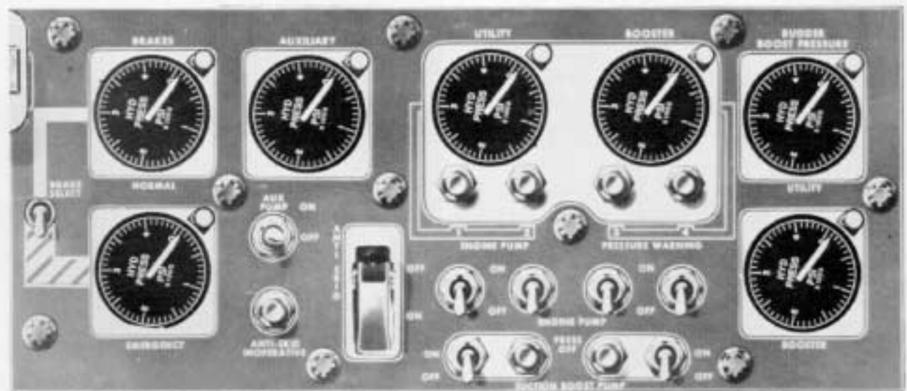
Hydraulic control panel – copilot's instrument panel.
