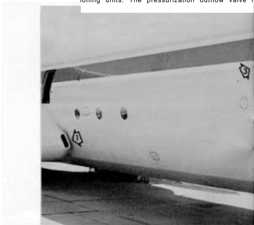
Right side view of L-100-30 shows inlets for (1) conditioning units. The pressurization outflow valve is
