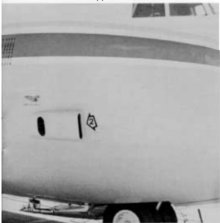
cargo compartment and (2) flight station air conditioning located behind the louvers (3).
