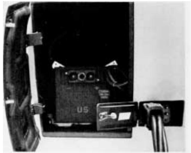
Onboard storage battery and external power receptacles-left side forward of crew entry door.
