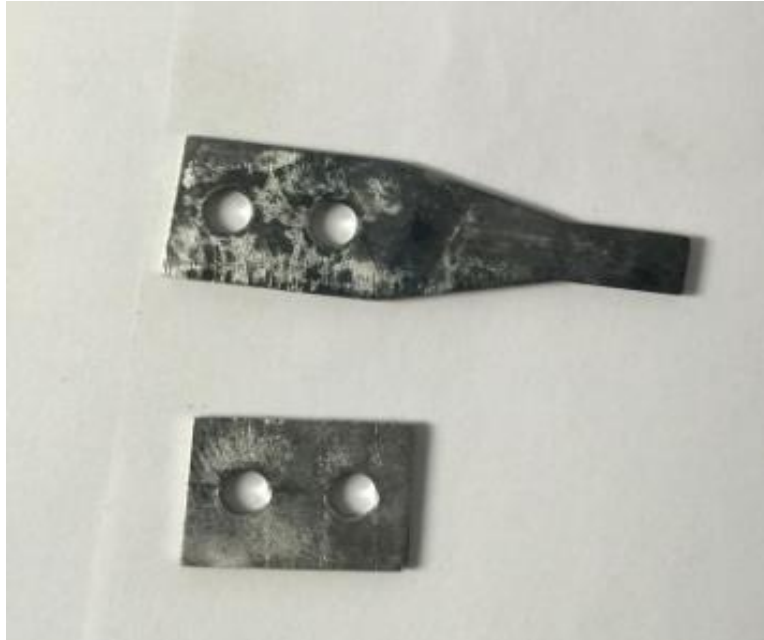
Figure 5 Improper chemical cleaning can cause additional problems.
