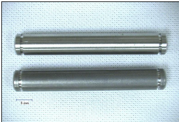
Figure 6 The bottom pin has aluminum oxide residue.
