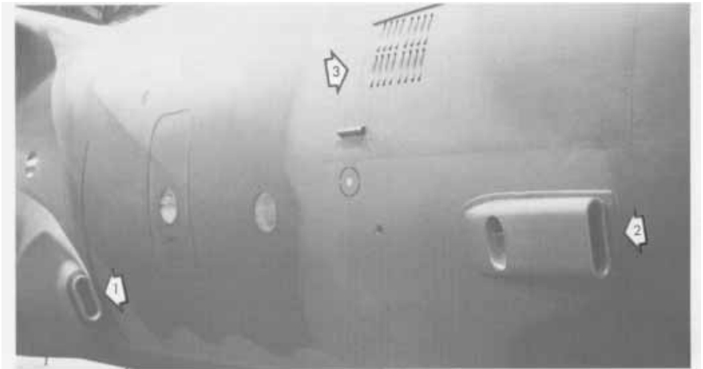
Right side view of L-100-30 shows inlets for (1) cargo compartment and (2) flight station air conditioning units. The pressurization outflow valve is located behind the louvers (3).
