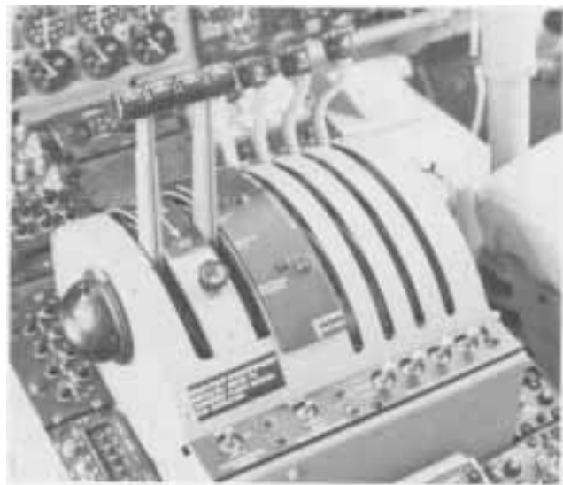
Engine control quadrant-flight station.
