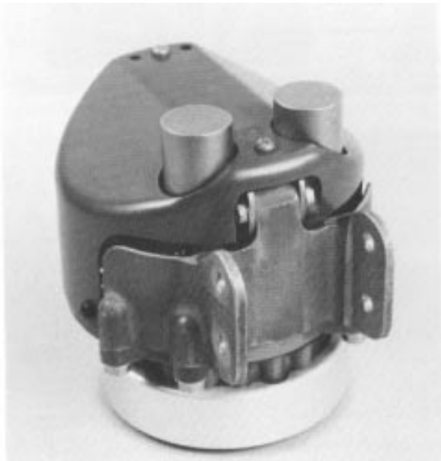
A dual level-control and shutoff valve (fill valve) is installed close to the top of each fuel tank.
