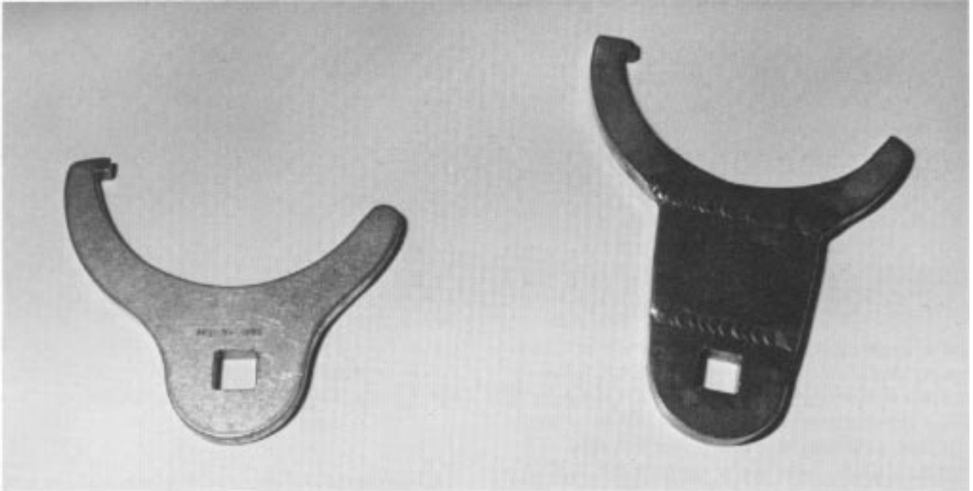
Figure 2. Unmodified (left) and modified 3600.48DH spanner wrench.
