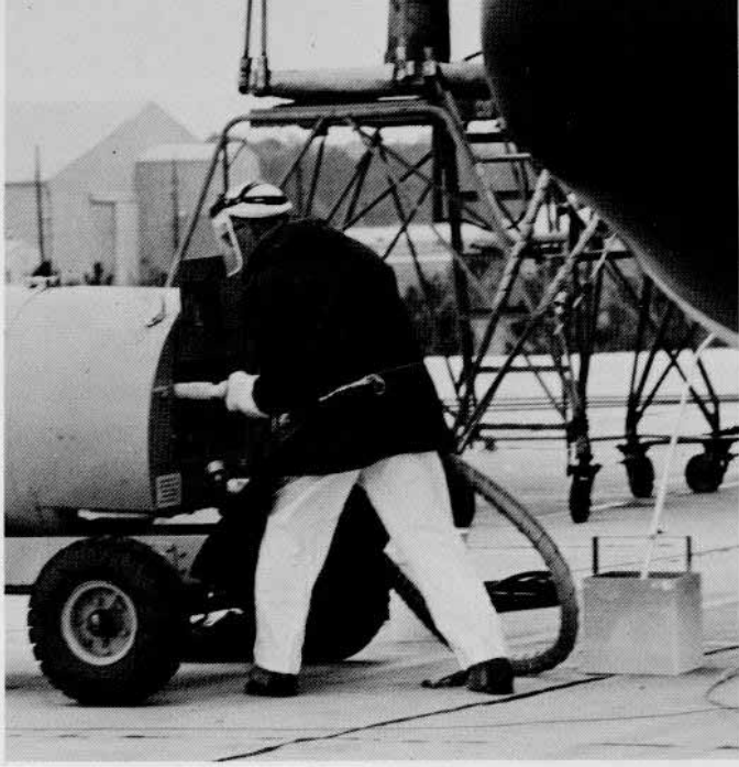
Purging the transfer cart system.
