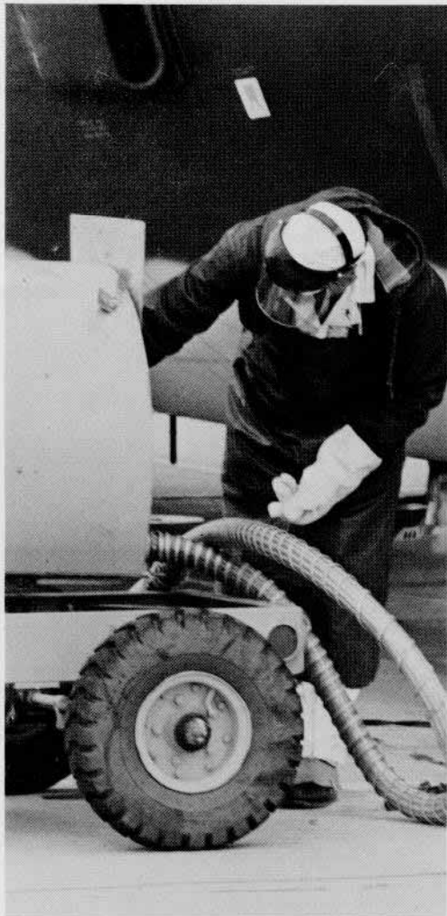
Installing the drain tube between the overboard vent opening and the drip pan.
