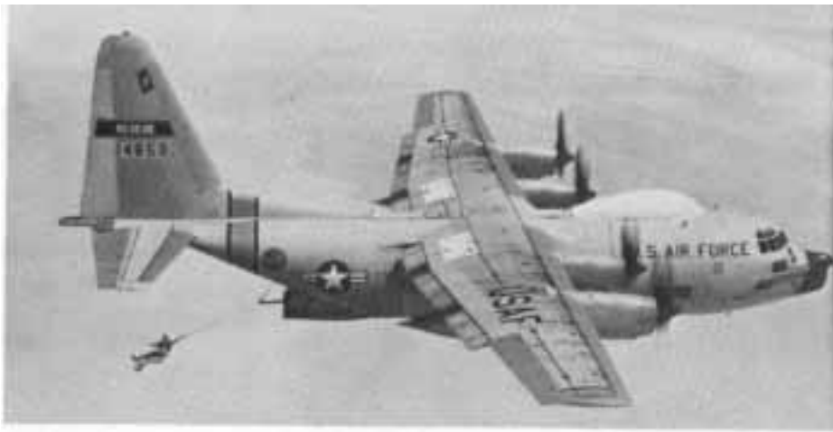
An Air Rescue Service Hercules demonstrates an inflight pickup of personnel from the surface.
