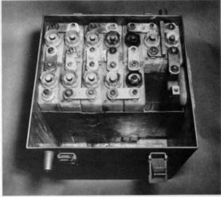
The photo at right shows what can happen when a nicad battery is allowed to deteriorate to a condition conducive to thermal runaway. Cells were removed to reveal a hole burned through a stainless steel divider. The photo at left shows cells with walls destroyed by a thermal runaway. Leaking electrolyte acted corrosively and acted as a conductor directly to the battery case.
