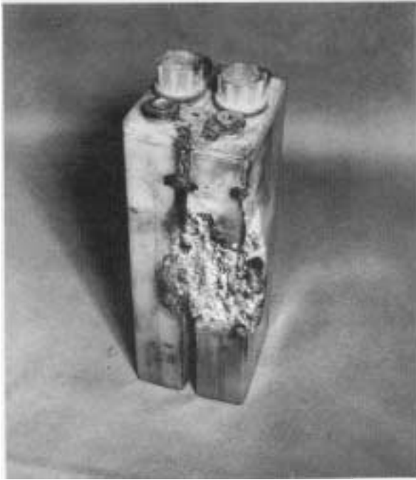
The photo at right shows what can happen when a nicad battery is allowed to deteriorate to a condition conducive to thermal runaway. Cells were removed to reveal a hole burned through a stainless steel divider. The photo at left shows cells with walls destroyed by a thermal runaway. Leaking electrolyte acted corrosively and acted as a conductor directly to the battery case.
