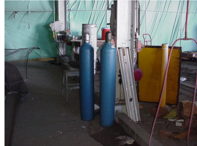
Gas Cylinders Not Secured
