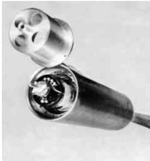
Figure 6-6 Typical Model and Roll Mechanism Assembly
