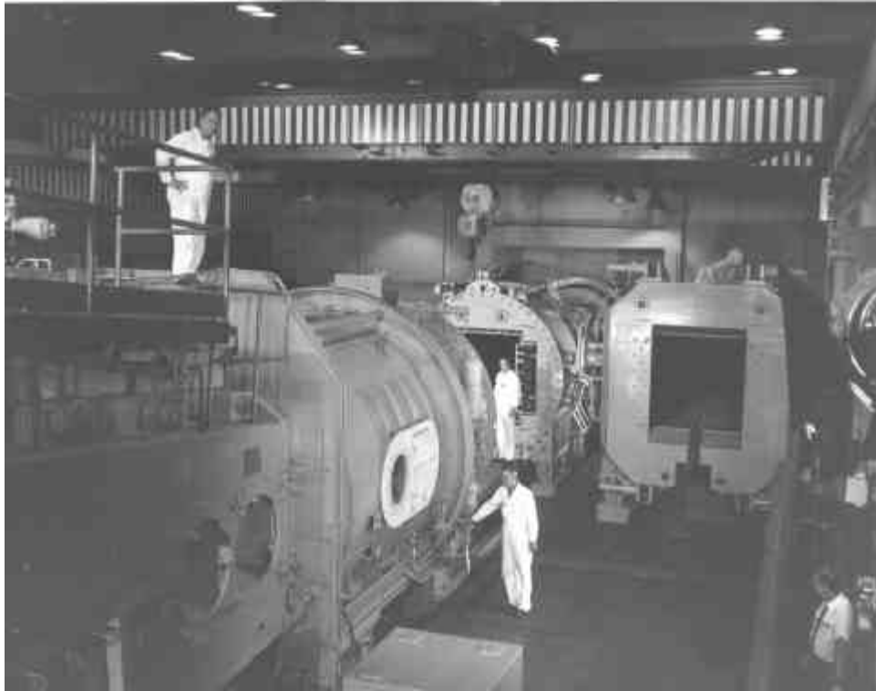
Figure 2-7 High-Bay Area with Transonic Test Section in Place
